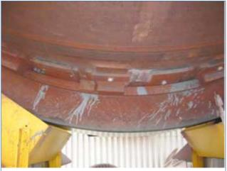
Figure 3. Wear pads in good condition.
