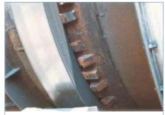
Figure 2. Wear pads in poor condition.
