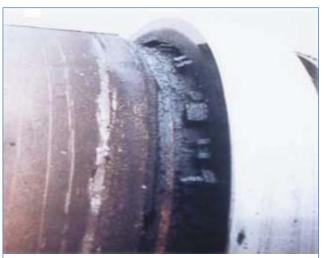
Figure 4. A kiln tyre coated with grease lubricant: note the collection of dust and debris that has contaminated the grease and the resulting sludge consistency of the lubricant.
